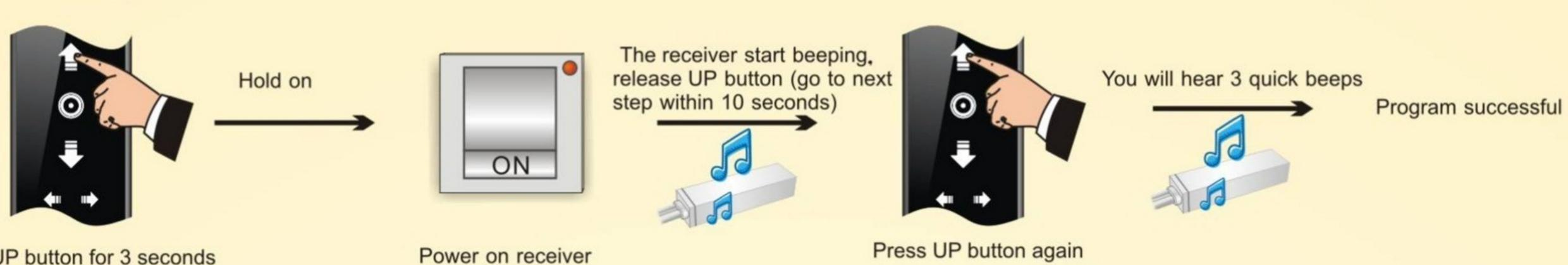
Press UP button for 3 seconds till LCD light is always light.
