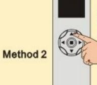
In dot move mode, press "UP" or "DOWN" on receiver shortly (<1.5s), motor will move dot by dot.
