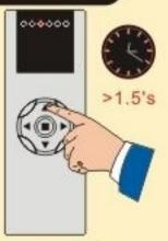
In dot move status, press "UP" or "DOWN" on receiver(>1.5s), motor will move continuously
