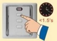
In dot move mode, press "UP" or "DOWN" on receiver shortly (<1.5s), motor will move dot by dot.
